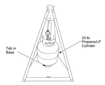
Figure 11 - Installing Propane/LP Cylinder
